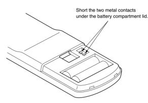
• To end test operation, press the remote control unit START/STOP (When the air conditioner is run by pressing the remote control unit TEST RUN button, the OPERATION and TIMER lamps will simultaneously flash slowly.)
