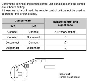
2. SWITCHING REMOTE CONTROL UNIT SIGNAL
